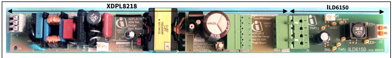
Figure 15 Modular reference design consisting of AC-DC converter based on XDPL8218 with ILD6150 DC-DC buck
