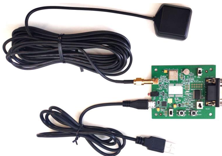
Figure 2: EVb and Accessories Assembly
