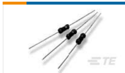
TE Part #5-1625890-2 2W SM M/OX 5% 47K
