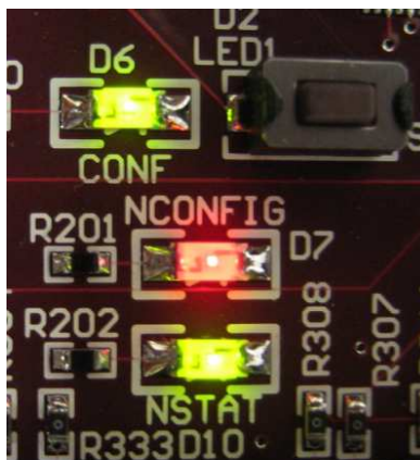
Figure 2-12. LED's at Power ON
