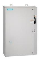
Non-reversing motor starter Size 1 Three phase full voltage Solid-state overload relay OLRelay amp range 0.25-1A 240VAC 50HZ / 277VAC 60HZ coil Combination type 30Amp non-fusible disconnect Encl NEMA type 4X 316 S-steel Water/dust tight non-corrosive Extra-wide enclosure
