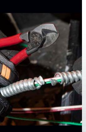
CUTS AND REMOVES ALUMINUM METAL CLAD (MC) CABLE JACKET
