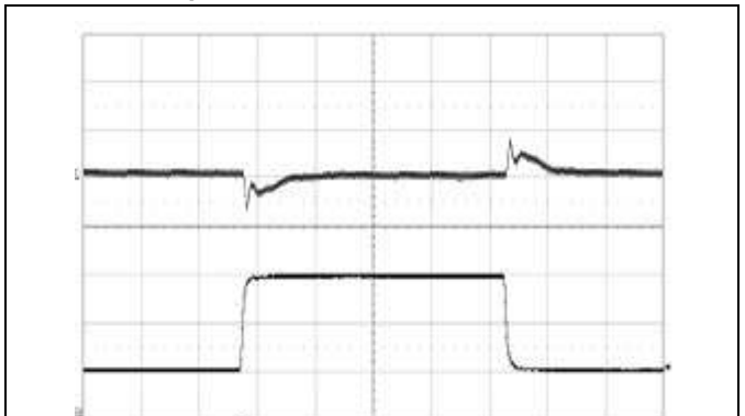
Output voltage response to load current step change (10–30–10 A), di/dt = 2\text{ A}/\mu\text{s} , at V_I = 12\text{ V} , C_{OUT} using standard test board Compensation settings by product /003 . Scale: 100 mV/div, 10 A/div, 500 \mu\text{s} /div.
