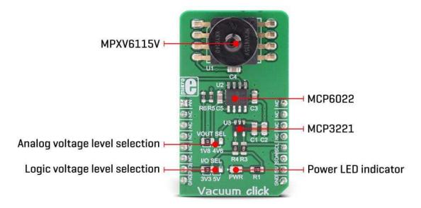
The sensor itself outputs about 4.6V DC voltage on its output pin when it is located at the sea-level pressure. As the pressure decreases, the voltage drops towards 0V. The internal circuit ensures that the voltage drop is linear with the pressure. The MPXV6115V datasheet offers a graphic diagram that shows the output voltage with respect to the applied pressure. It can be utilized for absolute pressure measurement, allowing the exact value of the pressure to be extracted.
