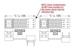
"A" = (No. of Conductors x 0.050 [1.27]) + 0.095 [2.41] "B" = (No. of Conductors -1) x 0.050 [1.27]
