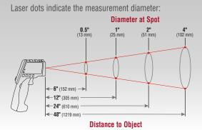
The IR5 dual lasers assist in targeting the measurement area. The distance between the two laser spots on the surface of the object being measured approximates the diameter of the circular measurement area from which the infrared sensor is collecting data.
