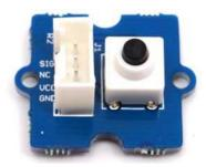
This new version of button Grove module contains one independent button, which are configured with pull-down resistor – ready for use with our microcontrollers as digital input. The button signals the SIG wire, NC is not used on this Grove module.
