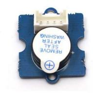
The Buzzer is a simple yet enjoyable Grove to use. It is piezoelectric speaker, coupled with a simple control circuit. If it is connected to a digital output, it will emit a tone when the output is high. Alternatively, it can be connected to an analog (really, pulse-width modulated digital) output to generate various tones and effects.
