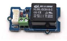
The Relay is a useful tool to magnify your Arduino's control ability! Feed the control signal through the Grove interface and the relay open or close the external circuit that is connected to the screw terminals. The voltage of the external circuit can run up to 220V! So grab this relay and start some really tough projects!
