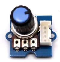
The Grove potentiometer produces analog output between 0 and VCC (3.3 or 5 VDC). The angular range is 300 degrees, with a linear change in value. The resistance value is 10k ohms, perfect for Arduino use. This may also be known as a "rotary angle sensor".
