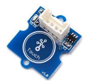
The Grove - Touch Sensor enables you to replace pressure on a button with contact on a detecting surface. It can detect the change in capacitance when a finger is nearby. So, whether your finger touches the pad directly or just stays close to it, the Grove - Touch Sensor would output HIGH.
