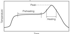
For soldering (Example: Sn/Pb)
