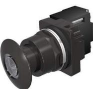
30mm BlackMax, Epoxy Coated Corrosion Resistant Complete Metal Unit Illuminated Push-Pull Operator Transformer type, 600V AC Incandescent Lamp Mushroom Head Cap Small 1 3/4" (44.5 mm) Metal, Black with Clear Lens 3 Position Pull-Momentary/Push-Maintained UL Listed, CSA Certified NEMA 1,3,3R,4,4X,12,13 & Automotive Standards
