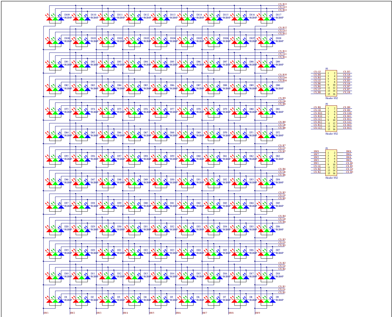
Figure 4: FxLED_9x13_ARRAY Application Schematic
