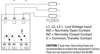
$! = \mbox{Select alarm contact connection as N.O. or N.C. when ordering; N.O. Shown.$
