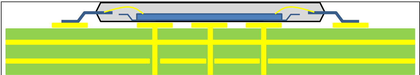
Figure 8-1: Example thermal via holes on PCB.
