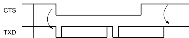
Figure 34-29. Transmitter Behavior when Operating with Hardware Handshaking
