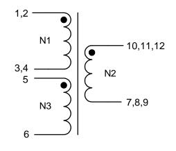
Application of the transformer allows for the leadwires between terminals 1&2, 3&4, 7&8&9, and 10&11&12 to solder bridge.
