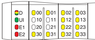
Figure 8 Local diagnostic and status indicators
