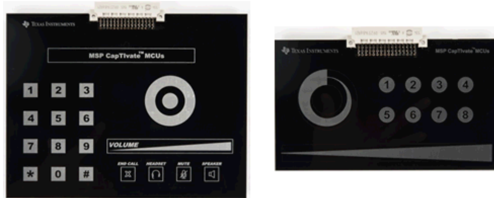
Figure 10-6. CAPTIVATE-PHONE and CAPTIVATE-BSWP Panels
