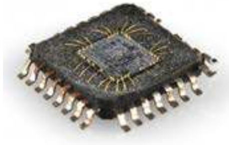
The guts of an integrated circuit, visible after removing the top.
