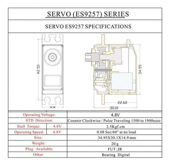
Note: This servo is recommended to use at 4.8V. (damage under higher voltage is not covered by warranty)
