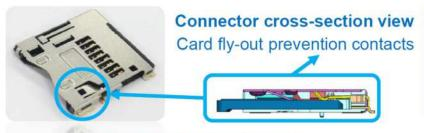
When ejected, Memory & SIM cards' ejection speed are reduced by the stopper contacts to prevent unexpected flyout motion.
