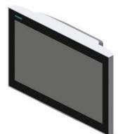
SIMATIC ITC1500 V3 PRO, Industrial Thin Client, 15" widescreen TFT display, capacitive touch sensor, Supported protocols: RDP, VNC, Smart Server, HTML5, etc., standard design, prepared for support arm with add-on elements
