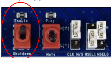
Figure 8. Left toggle switch set to “enable” position.
