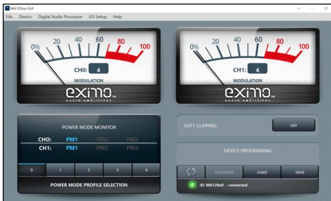
Figure 9. MA120xx control software interface
