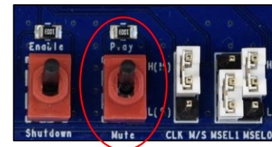
Figure 11. Right toggle switch set to “play” position.
