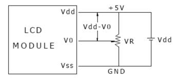
Vdd-V0: LCD Driving Voltage
