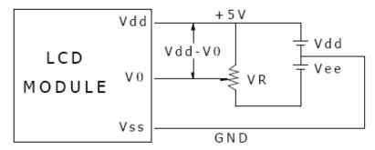
Vdd-V0: LCD Driving Voltage
