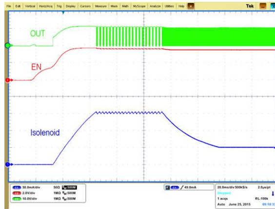
Figure 1. Solenoid Current, EN, and PWM vs Time
