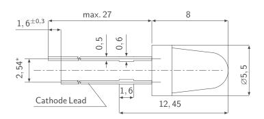
all dimensions in mm. Tolerance  $\pm 0,\,1$  except given ones \* at the bottom of the LED
