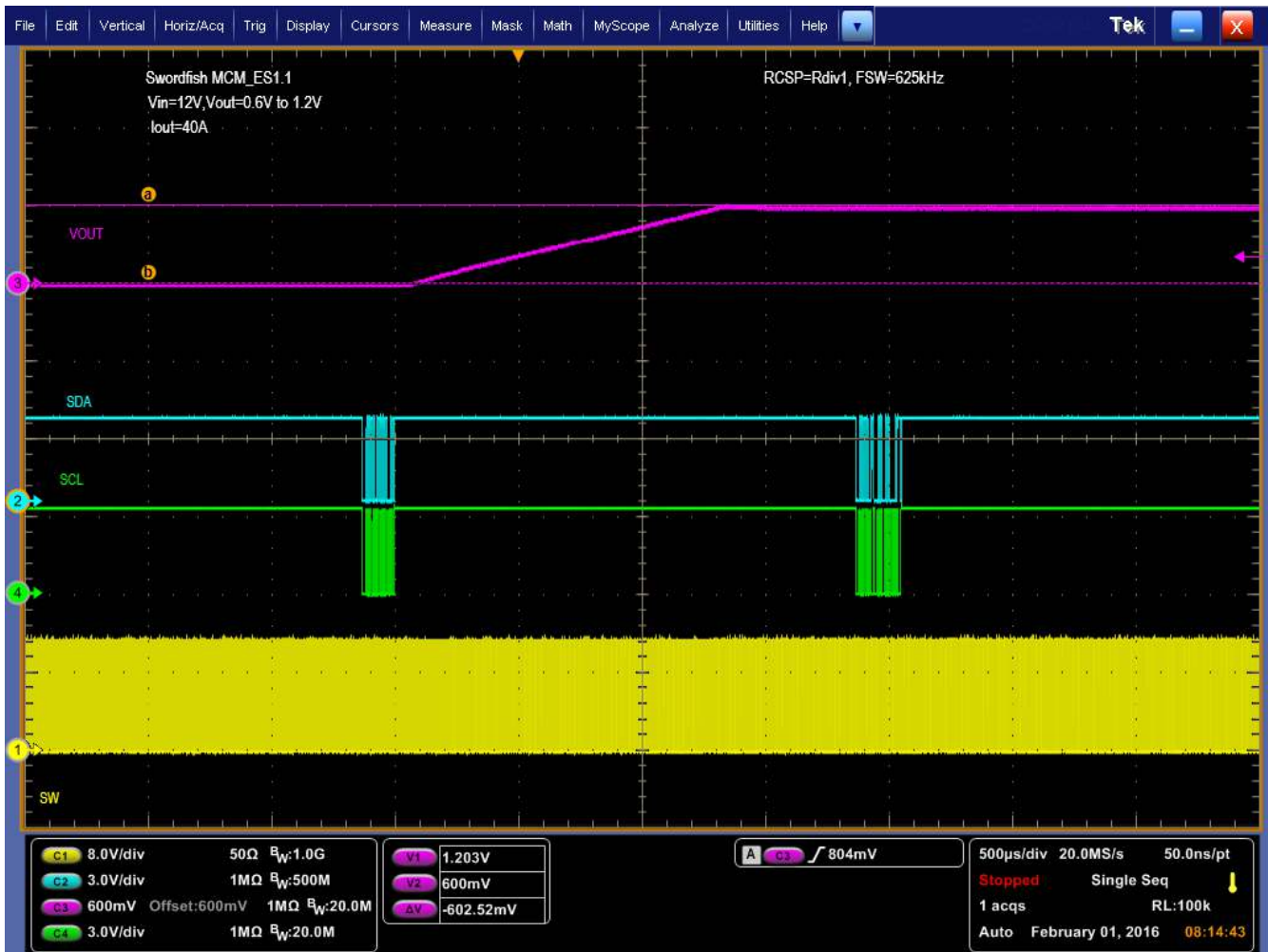
Figure 11-6. PMBus V_{OUT} Step-Up = 0.6 V to 1.2 V at 40 A
