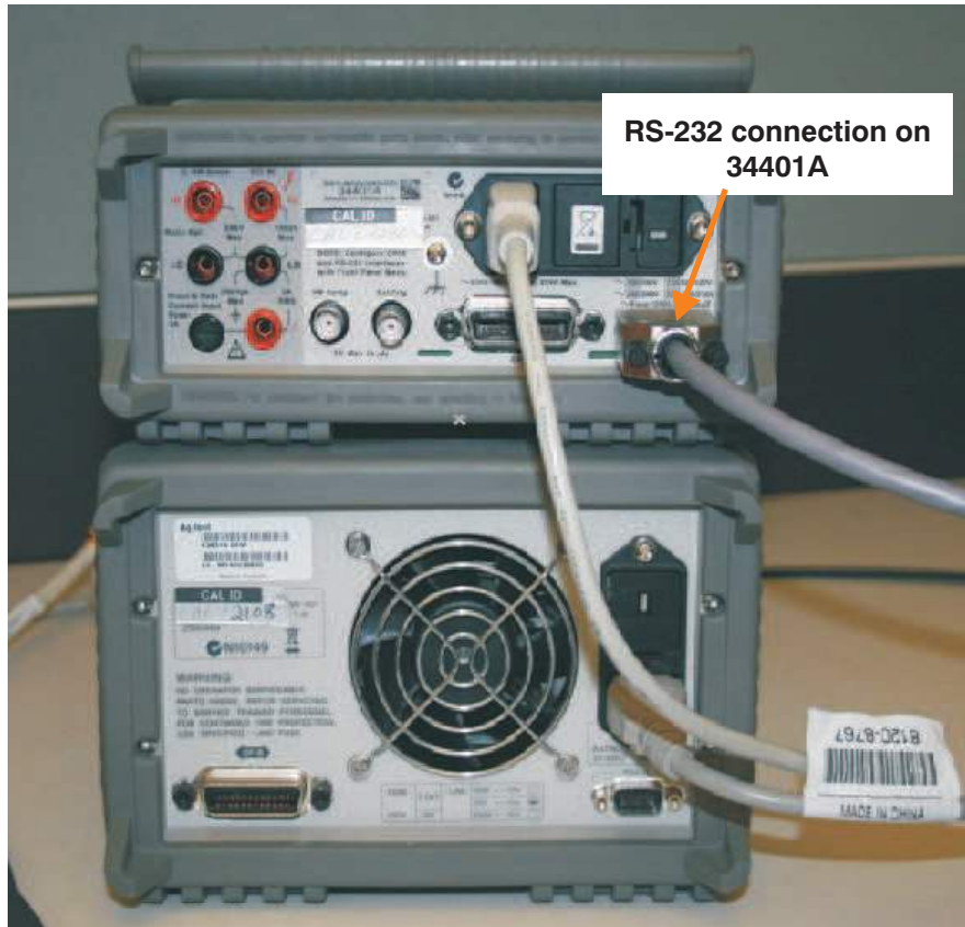
Figure 18. Connect Serial Port to DMM
