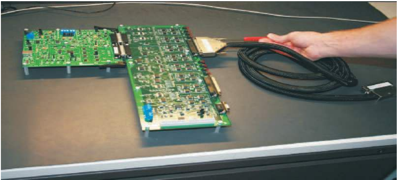
Figure 9. Connect Multi-Cal-Interface Cable to Multi-Cal-Master PCA Card
