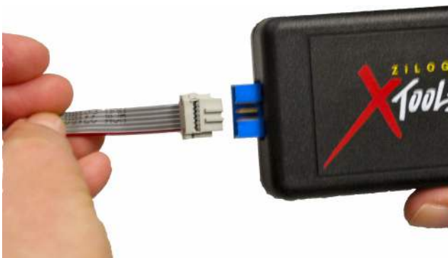
Figure 7. Connecting the Six-Conductor Ribbon Cable to the USB Smart Cable
