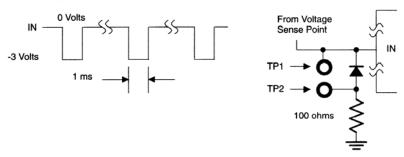
NOTE: This series of pulses must be applied during normal +5 volt operation.
