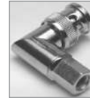
Right Angle, Twist-On BNC (M) 1 Piece, Solderless
