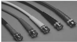
RG-59 Audio & Video BNC to BNC Cables Constructed of RG-59, 75 Ohm, 80% Braid, 22 AWG Stranded Cable, Matching Colored Boots & Cable.
