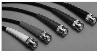
RG-58 Thin Ethernet BNC to BNC Cables Constructed of 50 Ohm, 95% Braid & 100% Foil Shield Cable, 20 AWG Stranded (Belden 9907 Equivalent), Black PVC Cable.
