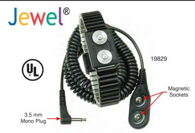
Jewel® MagSnap Wrist Straps meet or exceed the requirements of ANSI/ESD S20.20 and ANSI/ESD S1.1 including section 5.4 Breakaway Force "With the ground cord connected to the cuff in a normal manner, a force of  $\geq$  .45 kg (1 lb) but  $\leq$  2.3 kg (5 lb) applied to the ground cord, in the normal disconnect direction, shall be required to separate the ground cord from the cuff."
