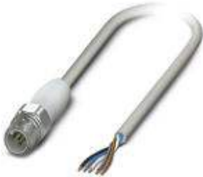
Sensor/Actuator cable, 5-position, PP-EPDM halogen-free, Gray RAL 7035, Plug straight M12, A-coded, on Free cable end, Cable length: 5 m, Hygienic design, With high-grade steel knurl
