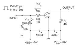
$I_{C}=10I_{B1}=-10I_{B2}=2A$ For PNP, the polarity is reversed.
