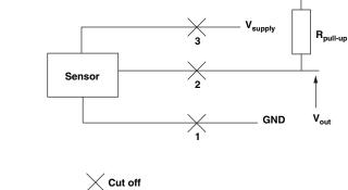
$V_{\text{pull-up}} \, \text{can be independent to} \, V_{\text{supply}}$
