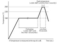
Temperature is measured at the top of a cell.
