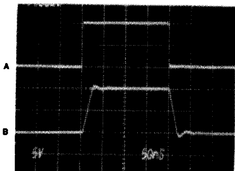
FIGURE 2. LARGE SIGNAL RESPONSE Vertical Scale: A = 0.5V/Div, B = 5.0V/Div. Horizontal Scale: Time = 50ns/Div.
