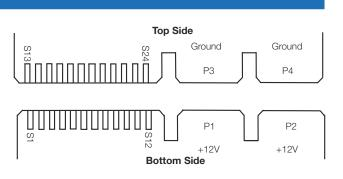
Note: Pin number may not necessarily match vendor's pin number assignment. Please follow the signal and number assignment as indicated in this datasheet  $% \mathcal{A}$
