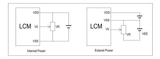
$V_{DD^{\sim}}V_0$ : LCD Driving voltage
