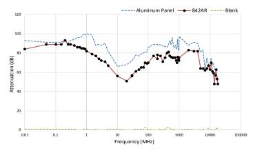
Test performed with a two-coat thickness.
