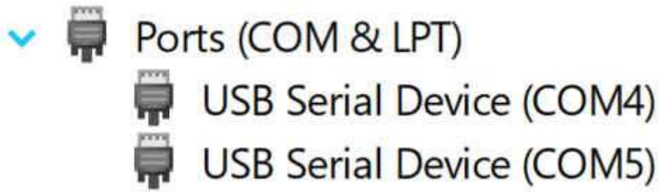
Figure 3-10. Typical Response After Connecting OPT4001YMNEVM to the Computer
