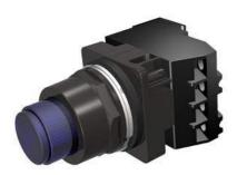
30mm BlackMax, Epoxy Coated Corrosion Resistant Complete Metal Unit PTT / Illuminated Pushbutton Full Voltage, 6V AC/DC Incandescent Lamp Extended Button Plastic Lens, Blue 2 Position Momentary with 1 N.O. - 1 N.C. Heavy Duty Contacts, A600/P600 UL Listed, CSA Certified NEMA 1,3,3R,4,4X,12,13 & Automotive Standards
