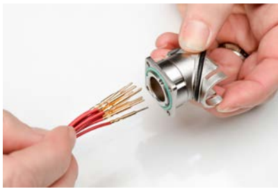
Step 3 - Side wires through shell
