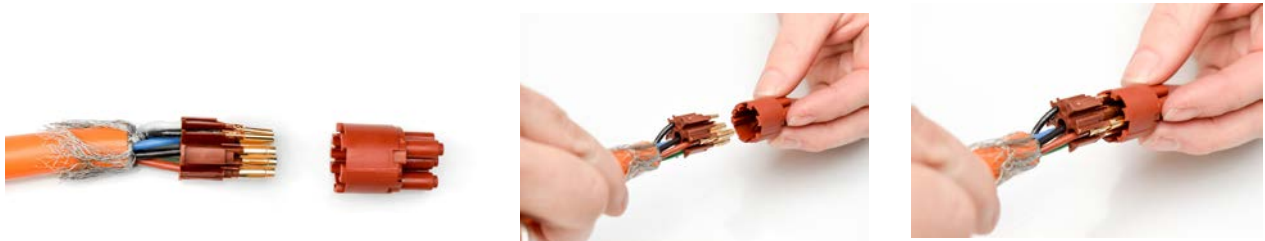
Step 11 - Push the contact holder into the sleeve
