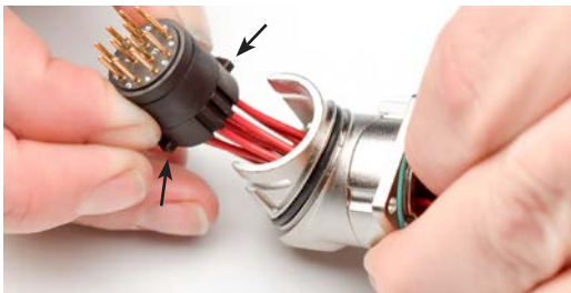
Step 5 - Locate keys on sides of insert
