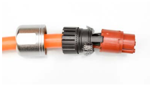
Step 13 - Clip the cord grip as shown with the shield sticking out around it
