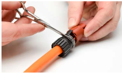
Step 14 - Trim shield as shown
