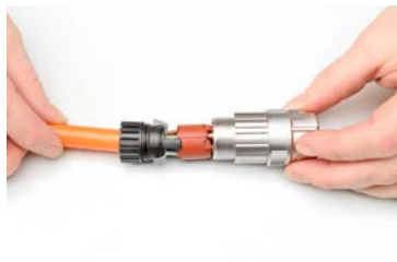
Step 15 - Push sub-assembly into shell
