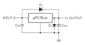
$C_{\text{IN}}$ : Required if regulator is located an appreciable distance from power supply filter (More than 2.2  $\mu$ F).
