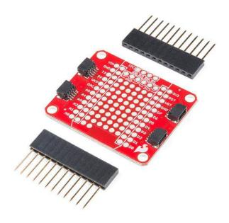
The SparkFun Qwiic Shield for Photon is an easy-to-assemble board that provides a simple way to incorporate the Qwiic Connect System with your Particle Photon. This shield connects the I<sup>2</sup>C bus on your Photon to a series of SparkFun Qwiic connectors. As long as your devices are on different addresses, the Qwiic system allows for daisy chaining, meaning you can stack as many sensors as you'd like to create a tower of sensing power!
