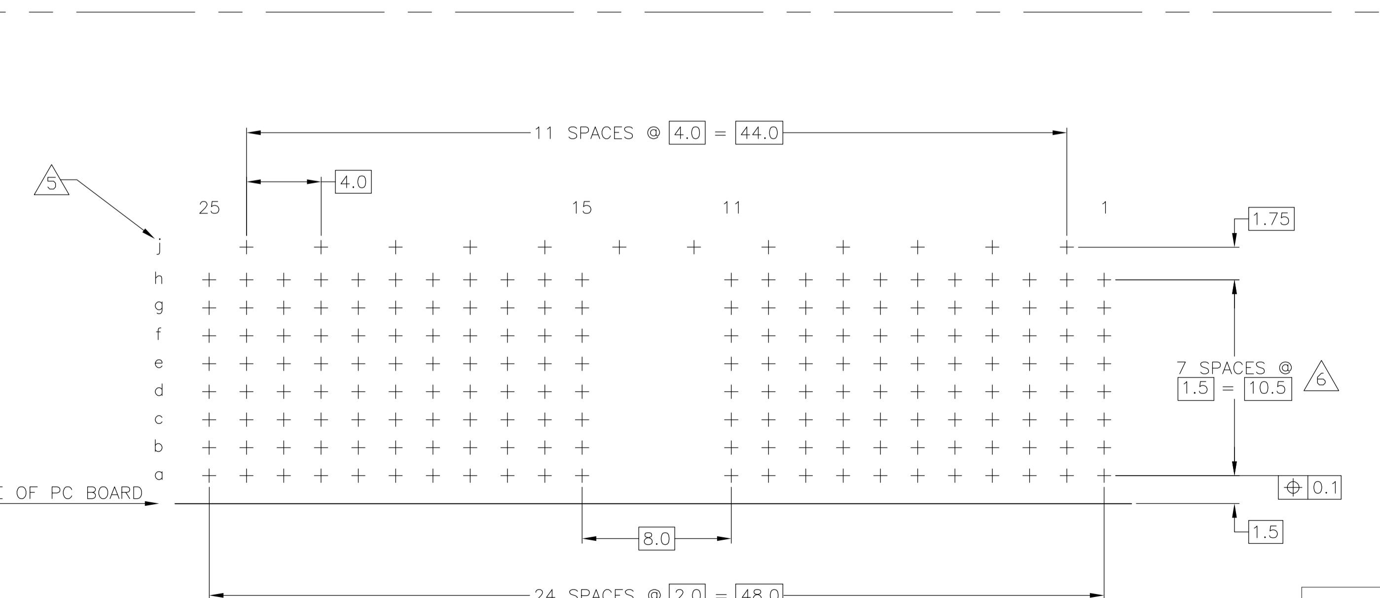
PCB HOLE DIM ACTION PIN
