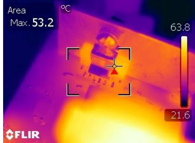
Figure 58 – Full Load HiperLCS Thermal View, Room Temperature.
