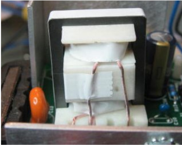
Figure 49 – Visible Light Transformer Front View.
