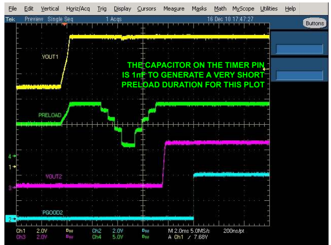
FIGURE 13. NORMAL POWER-UP SEQUENCE
