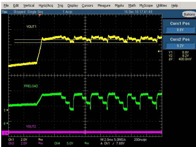
FIGURE 14. SOFT-START WHEN PRELOAD TEST FAILS
