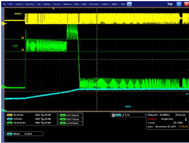
FIGURE 10. VR1 SOFT-START (FROM TOP TO BOTTOM: PHASE1, I L1 , V OUT1 )
